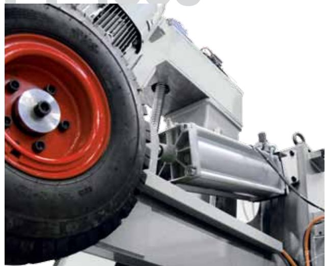
Portal take-up drive wheel Max reel weight 40 tons
