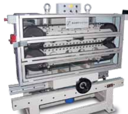
Mobile caterpillar for wire torsion locker for SZ process
