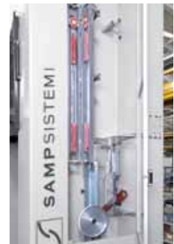
IN 1100 Close-up of the built-in dancer and cooling system for the hard wire and aluminium production
