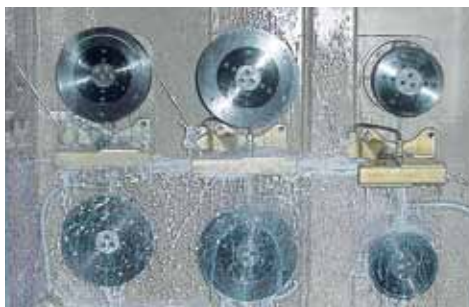
Spray or spray + submerged type lubrication can be provided
