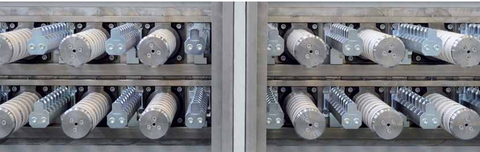
Close-up of the drawing area with 80 mm diameter drawing rings
